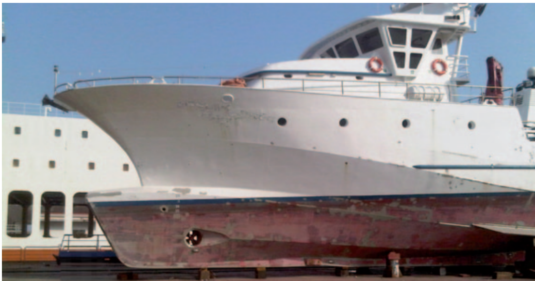
Figure 14.7 - Optimum integration of a bow bulb on a hull designed ex novo .
