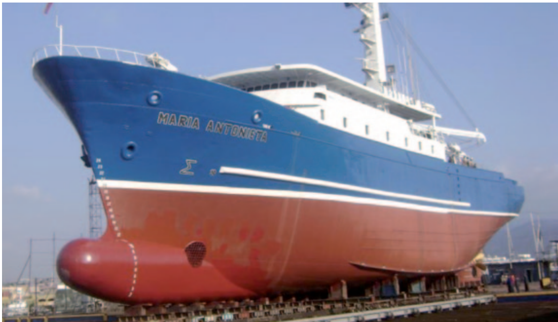
Figure 14.6 - Converting an existing hull by adding a bow bulb.
